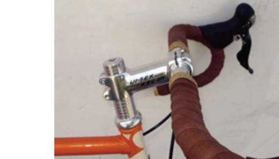
steel steerer lets you raise the bar much higher than a carbon steerer does. Still, not your grandad's bar-stem rig.
