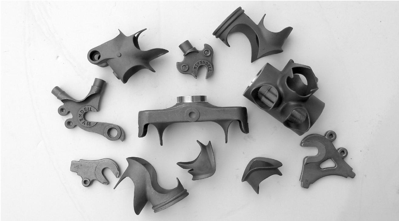
The Hunqapillar, like all of our bikes, is made with fine, strong, precision cast or forged lugs, dropouts, bottom bracket shell, and fork crown. Most of the fittings you see here are made just for us, and three of them were made just for the Hunqapillar. (Although we may use them on other models, when they make sense.) They're all steel, just like the Hunqatubes.
