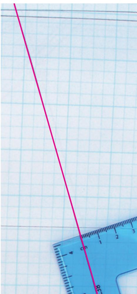
On this fork I picked a rake of 52mm, which, divided by four, is 13mm. So you get your Helix brand triangle with the metric graduations marked on it, and make the right-angle line between the fork's centerline and the center of the dropout whatever fork rake you want, divided by four.
