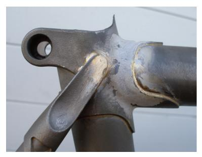
Seat lug. This one has an external seat stay cap, and horrors, it's not even our proprietary model. IT's still cast, still made by the same...and apparently it's a better fit with the double-tapered seat stays (thickwalled) than our plug is. So, we'll go with it. Prolly.
