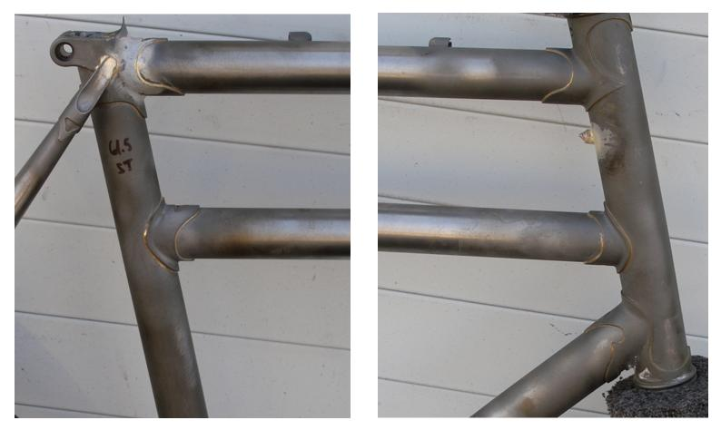
This shows the new lugs used for the second TT. Up to now, they've been made by carving up other lugs. This way is no better, but way less hassle, makes more sense. I like the gangly arm-y look of big bikes with relatively skinny tubes. Structually, it makes sense. The wall tubes don't have to be so thin to save weight. That makes them more prone to denting. These are thin enough.
